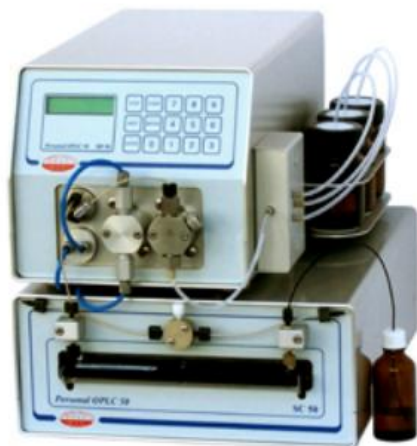
Rys. 5. Zestaw do OPLC firmy MicroSolv – Personal, OPLC 50 (MicroSolv Technology Corporation, Eatontown,USA) [81]
